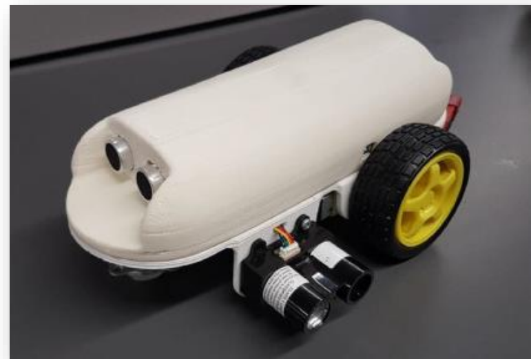
Robot ‘Dogs’ to keep shop floor clear of Foreign Object Debris.
