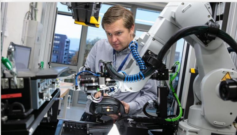
Robotic arms test cockpit instruments.
